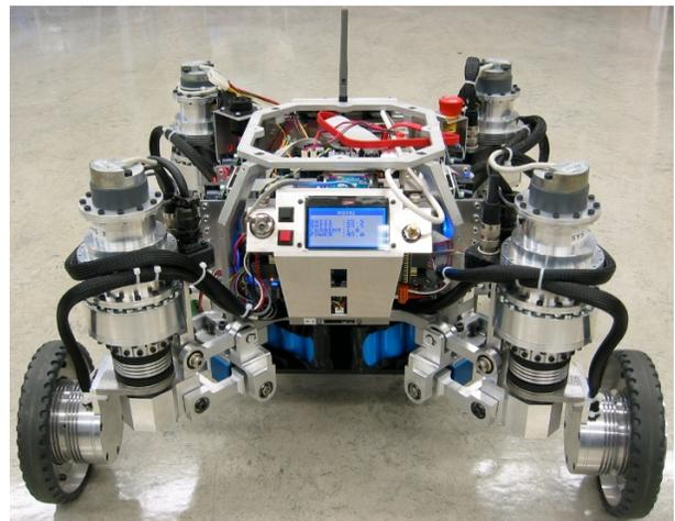
Fig. 1. AZIMUT-3 platform in its wheeled configuration
