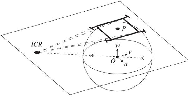
Fig. 2. ICR representation for AZIMUT-3. The chassis' center,  $P$ , is located at the zenith of the unit sphere, or  $(0; 0; 1)$ . The crosses represent the antipodal points which represents the ICR on the sphere.
