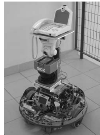
Fig. 5. Telerobot, the telepresence robot for home care assistance.
