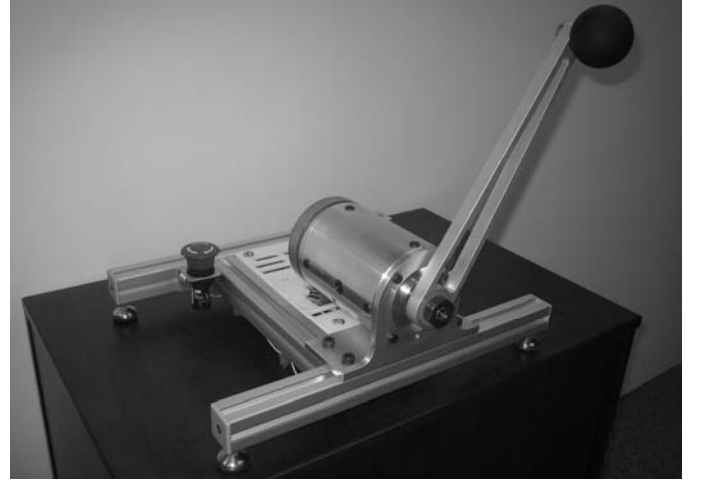
Fig. 19 Actuator with manipulandum acting as an inertial load.
