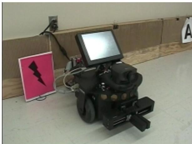
**Figure 7: Lolitta H, our Pioneer 2 robot that participated in the AAI’2000 Mobile Robot Challenge. The robot is shown next to the charging station symbol, and is docked for recharge.**
