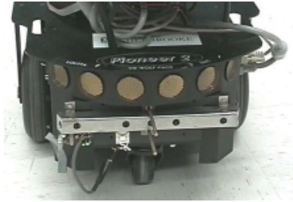
Figure 4: Back of the robot, showing the infrared ring.
