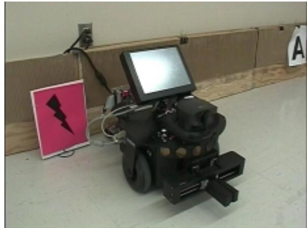
Figure 6: Lolitta H, our Pioneer 2 robot that participated in the AAI'2000 Mobile Robot Challenge. The robot is shown next to the charging station symbol, and is docked for recharge.
