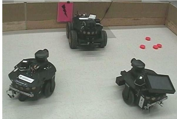
Figure 3: Group experiments having robots share one charging station.
