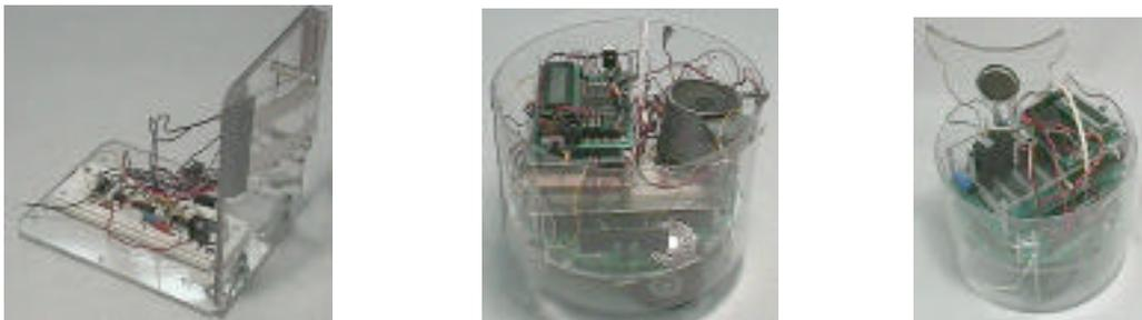
Figure 5. ROBUS equipped with a ISD ChipCorder (center) near a charging station (left), and with a sonar mounted on top of a servo-motor (right)
