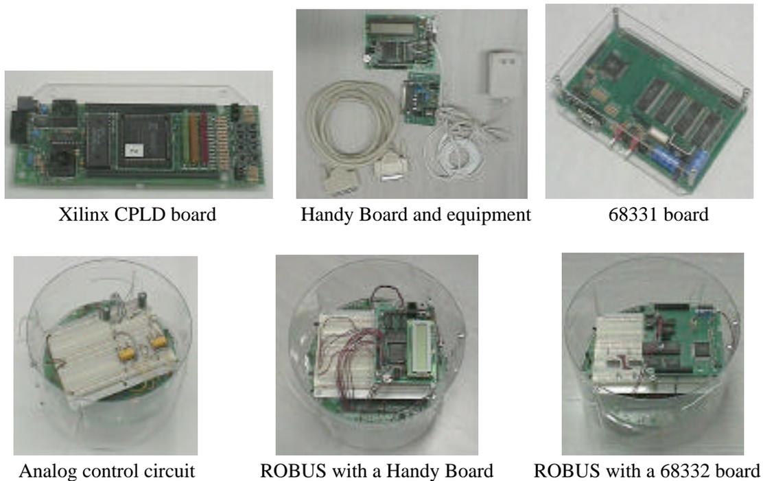
Figure 3. Control devices for ROBUS
