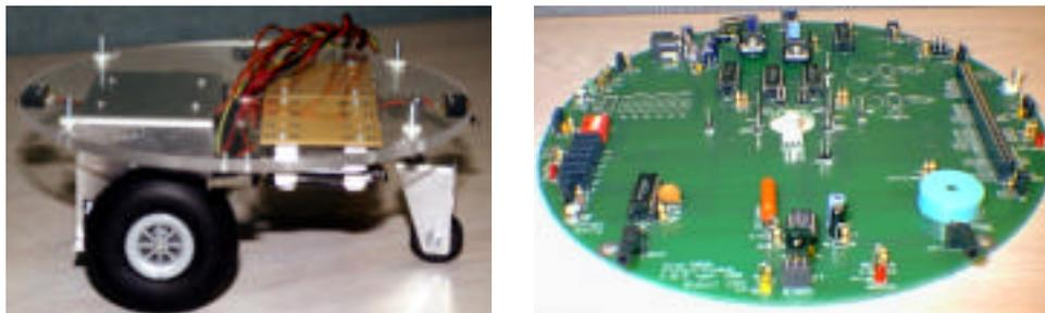
Figure 2. *Electro-Mechanical Base and Interface Circuit Board of ROBUS*
