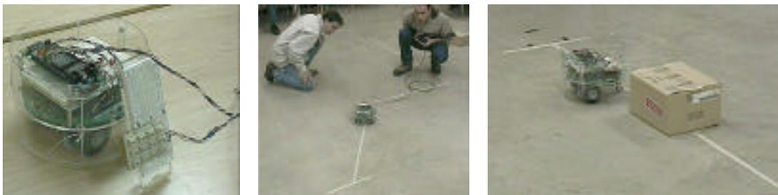
Figure 4. ROBUS used with the Xilinx CPLD board in the Logic Circuits course
