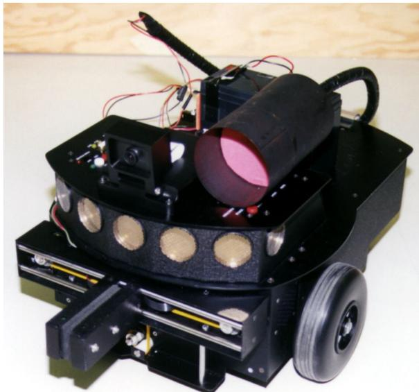
Figure 1: The Pioneer I robot used in our experiments, equipped with the visual signaling device on the right, next to the camera.
