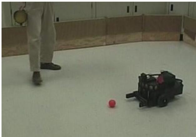
Figure 4: Ball-passing game between a Pioneer I robot and a human interlocutor.
