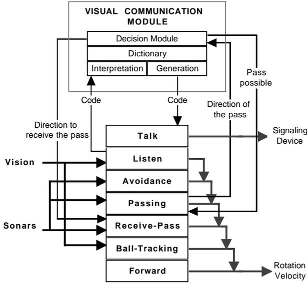
Figure 2: Approach used for ball-passing using visual signaling. Gripper control is done by *Passing* and *Ball-Tracking* and is not represented on this figure.
