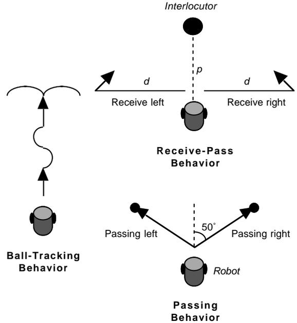
Figure 3: Trajectories generated by *Passing*, *Receive-Pass* and *Ball-Tracking*.
