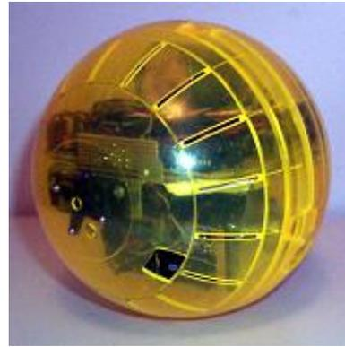
Figure 1: Roball, an autonomous rolling robot.
