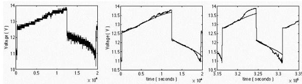
**Figure 5:** Samples of charge and discharge curves for a robot operating continuously for 94.4 hours.
