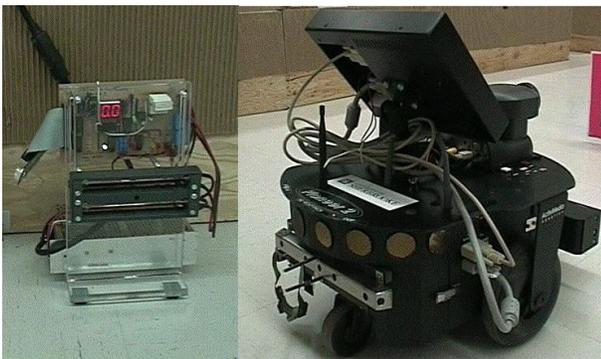
**Figure 1:** Our charging station (left), with one robot (right) seen from the back, with the IR detectors.
