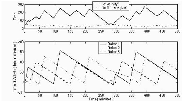
**Figure 4:** Graphs representing an experiment with three robots and with one power source, with  $T_A = [150, 120, 100]$ ,  $T_W = [300, 240, 200]$ ,  $T_C = [20, 15, 20]$ , and  $toa = [10, 30, 10]$ .
