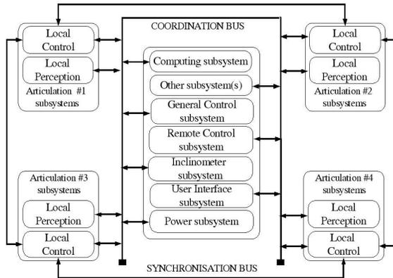
**Figure 5:** AZIMUT'S Hardware Subsystems.
