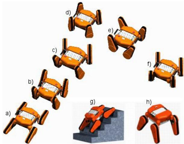
*Figure 2: Locomotion modes of AZIMUT.*
