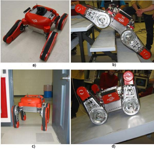
**Figure 7:** AZIMUT a) with its articulations stretched; b) on stairs; c) going through a door; d) on an incline surface.
