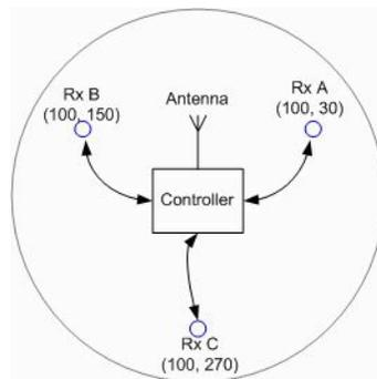
**Figure 3:** Disposition of the receivers Rx (A, B, C) and the controller with its RF link.
