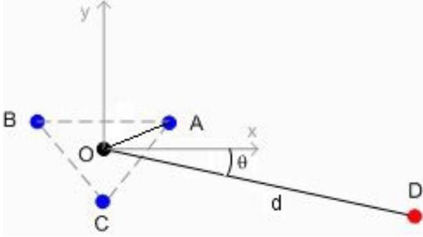
**Figure 1:** Three fixed receivers (A, B, C) and one transmitter (D).
