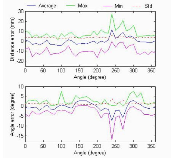
Figure 6: Errors in distance (top) and angle (bottom) from  $0^\circ$  to  $360^\circ$ , over 500 mm to 8100 mm.
