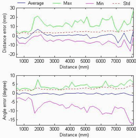
Figure 5: Errors in distance (top) and angle (bottom) from 500 mm to 8100 mm over  $360^\circ$ .
