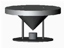
**Figure 2:** Reflector cone on top of a transducer, making it omnidirectional.
