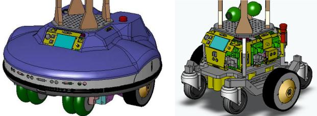
Fig. 6. Concept for the robotic platform, with and without bodywork.
