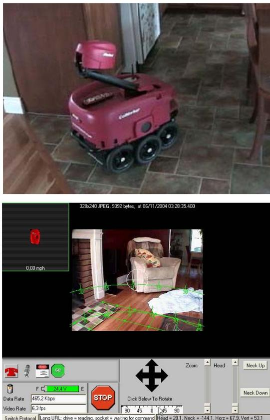
Fig. 1. CoWorker robotic platform (top) and its user interface (bottom).
