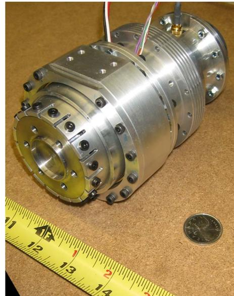
Fig. 2 – Differential Elastic Actuator
