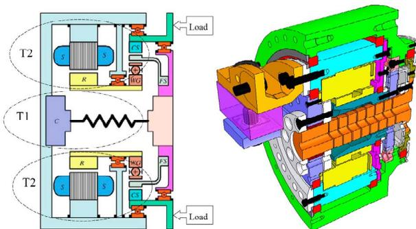
Fig. 1 - DEA implementation using a harmonic drive, a torsion spring and a brushless motor.
