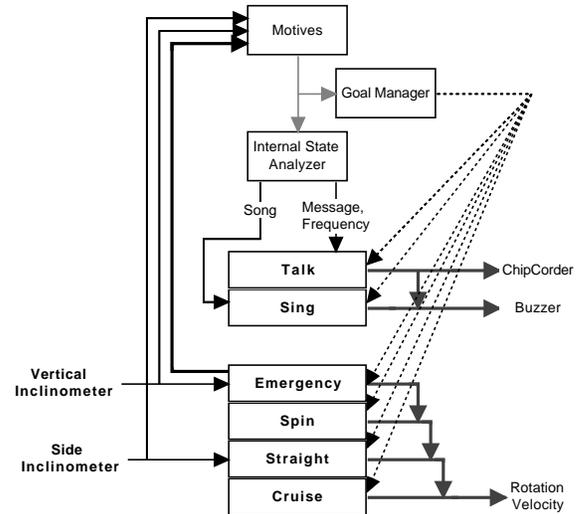
Figure 4: Decision modules used to control Roball.
