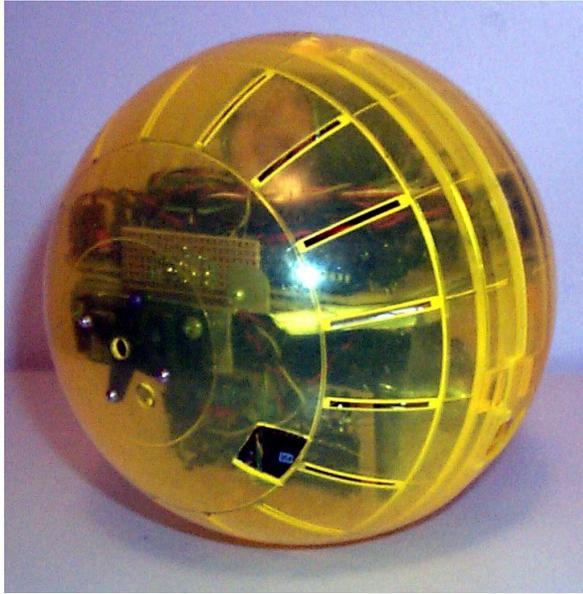
Figure 3: First prototype of our spherical robot.
