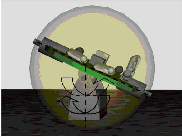
Figure 1: Rear view of the propulsion and steering mechanisms, as the robot turns to the right.
